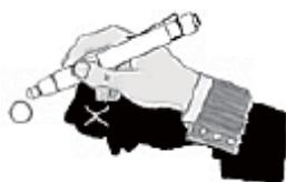
The writing angle between the pen tip and the screen should be less than 75°
