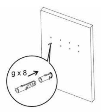
Step 5: Use PART F and PART E to make the PART A on the wall with 8 holes.
