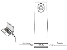
(1) Connect the power adapter to the video conferencing equipment and press the power button to turn on the device. The light ring lights up and the running light indicates that the device is booting up. A prompt tone is played when the boot-up is complete. <sup>(2)</sup> Connect the USB cable to the computer and press the mode switch button to select the desired display layout to output.
