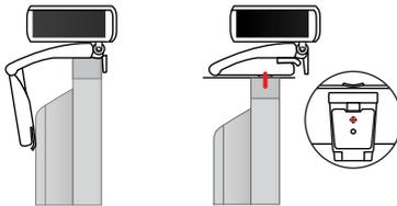
**Option 1:** use the articulated clamp to tighten to the screen edge
